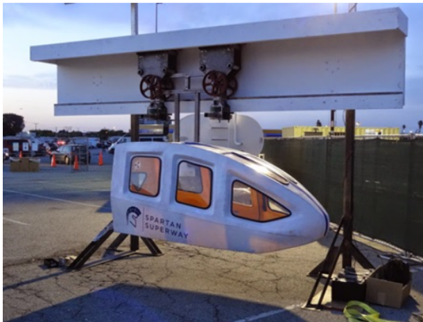
Figure 1 A prototype of ATN vehicle developed in SPARTAN Superway Project (see online version for colours)
