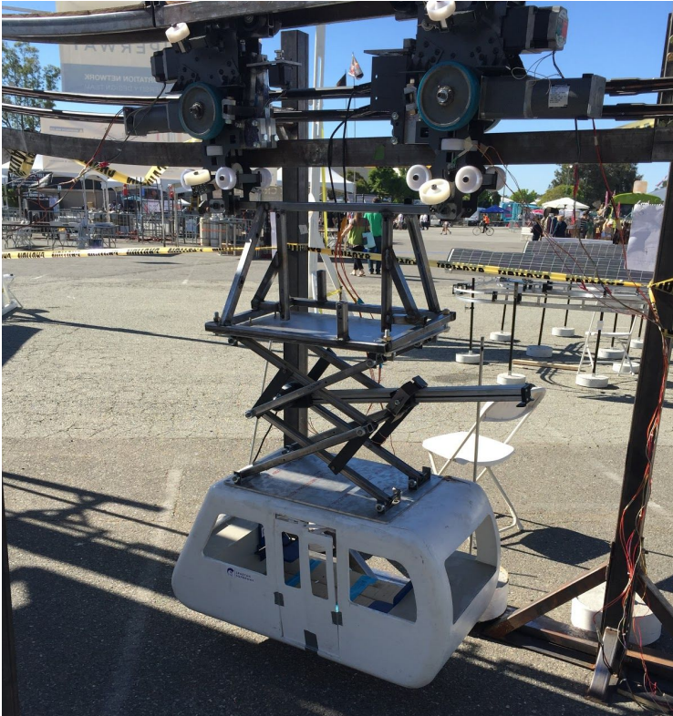
Figure 34: The stretchable shelf design for the control box from the previous team
