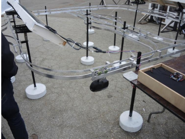
**Figure 4: 1/12<sup>th</sup> scale podcar and guideway system.** A small-scale prototype of the Spartan Superway allows for testing and analyzation to achieve full-scale optimization.
