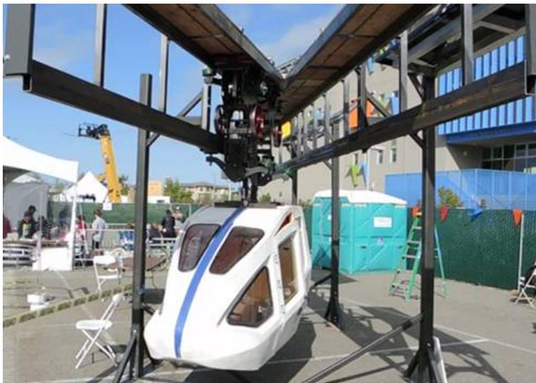
**Figure 5: Full-scale Spartan Superway model.** This full-scale model allowed the mechatronics team to create a switching mechanism to allow the podcar to travel along different railways.
