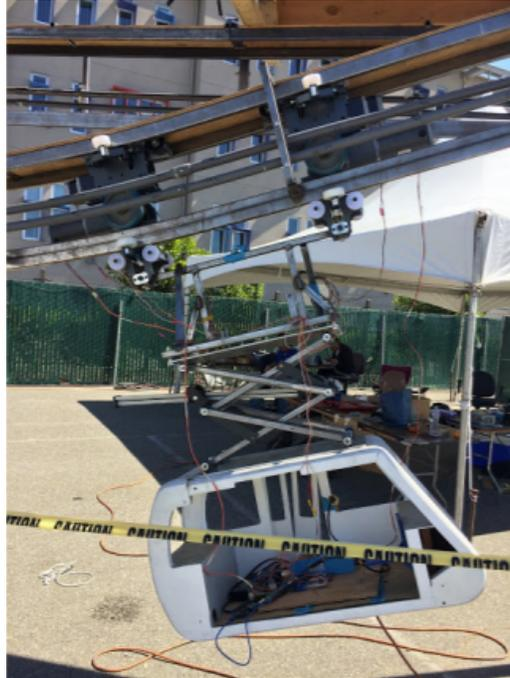
**Figure 6: Half-scale Spartan Superway Model.** The half-scale Spartan Superway model featured a scissor mechanism that allowed the podcars to pick up passengers on a street level.
