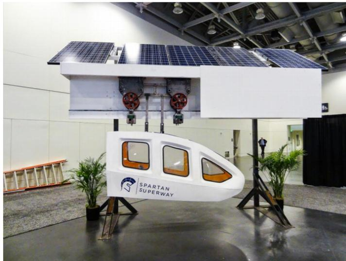
**Figure 1: Spartan Superway demonstration prototype.** This prototype depicts the many technologies the Spartan Superway plans to implement such as its solar panels, personal pedestrian podcar, and an elevated infrastructure.
