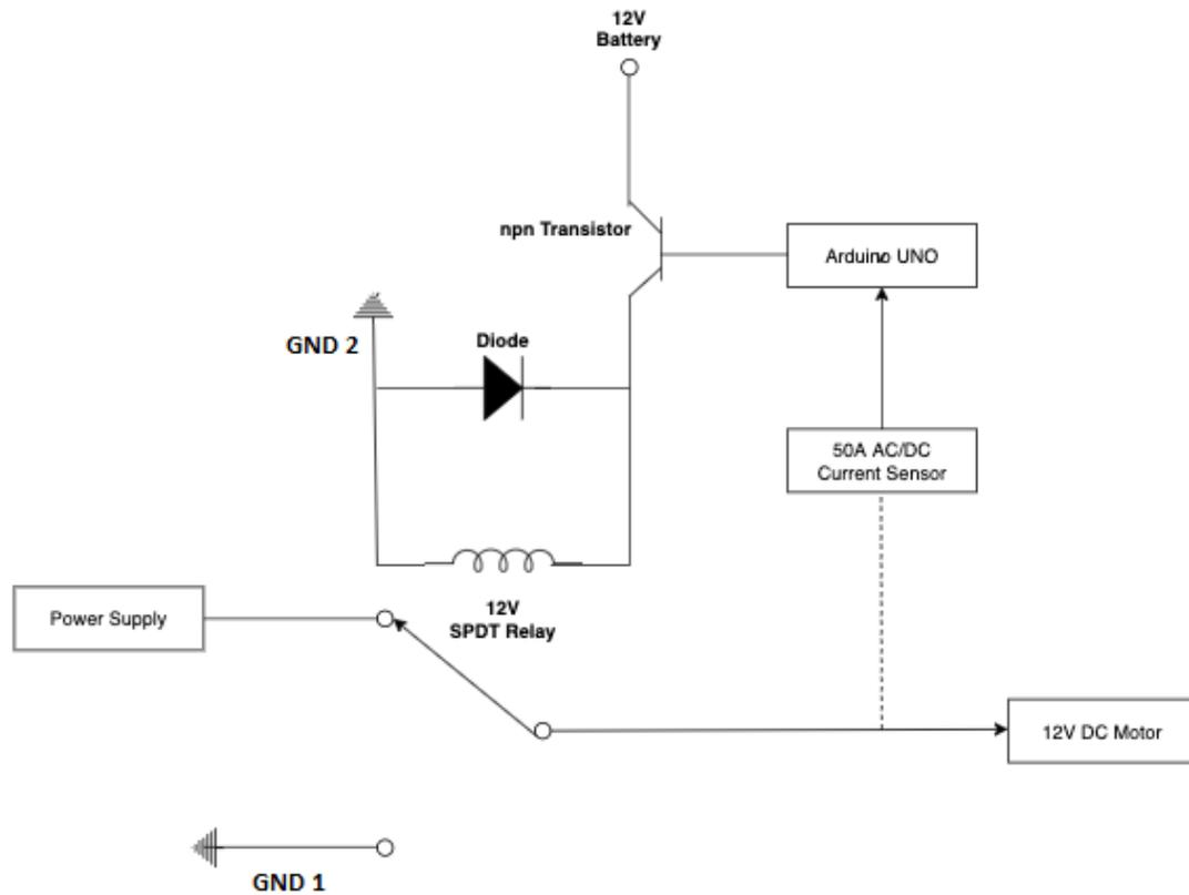
*Figure 26: 2-D simplified electrical schematic of the switching mechanism.*
