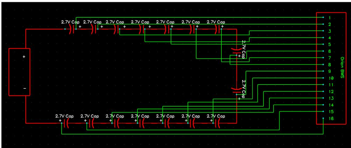
Figure 14: PCB schematic with 16 supercapacitor cells in series and connected to a BMS in P-CAD.
