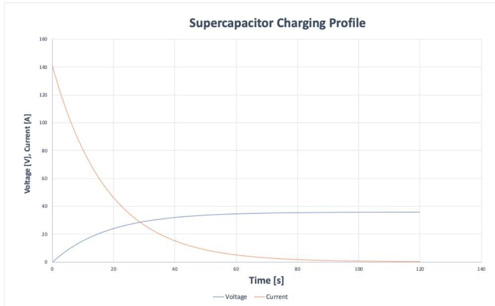
Figure 6: Charging Profile of Full-scale Power Module.
