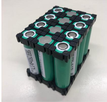
*Figure 7: Small Scale Lithium-ion Battery Pack.*
