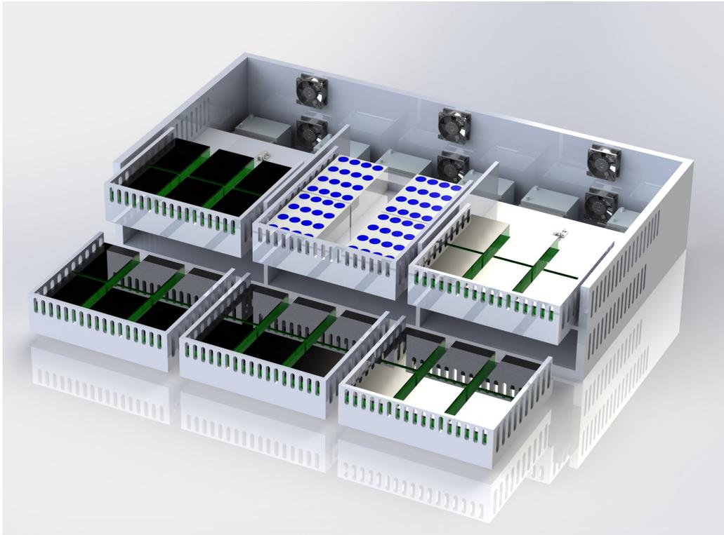
*Figure 23: Double-layered Power Module.*
