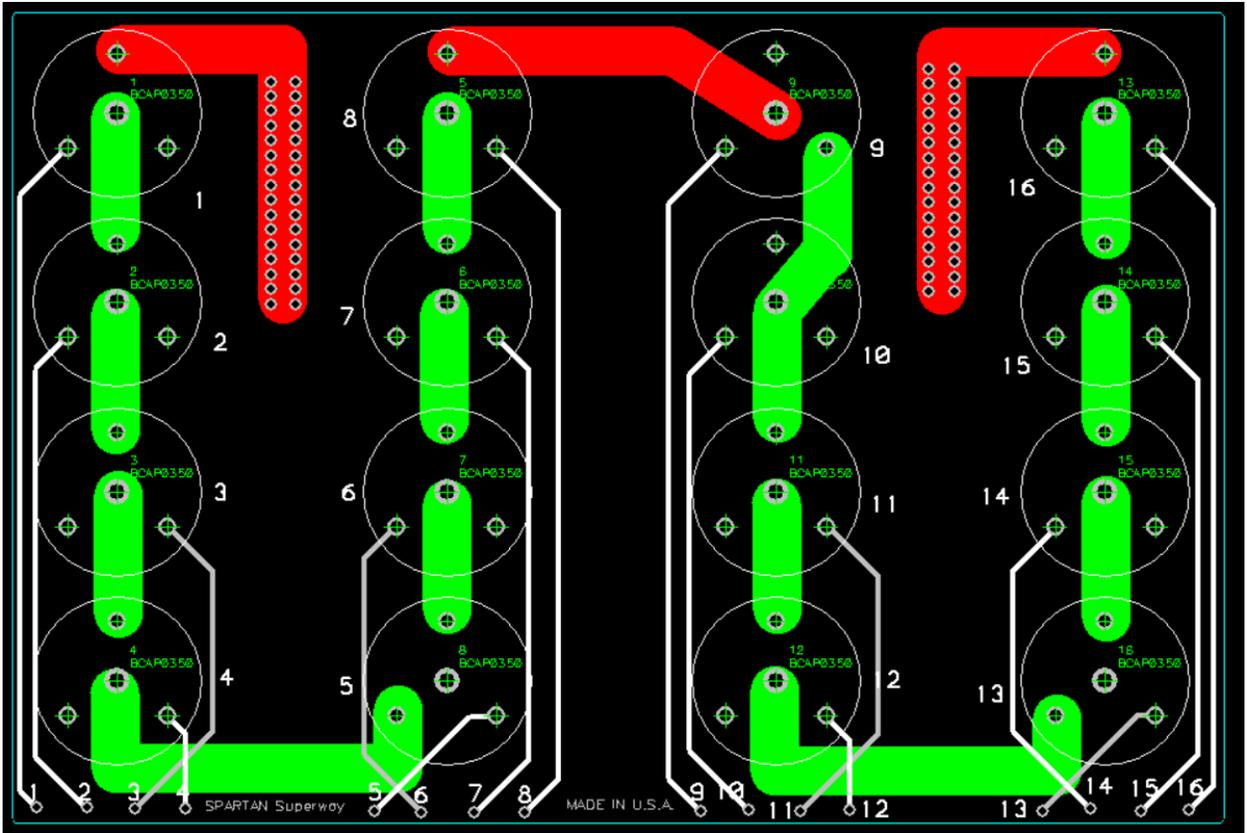
Figure 15: Final PCB design to handle 50 Amps.
