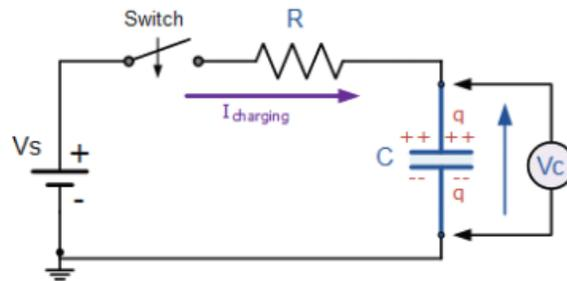
Figure 4: Supercapacitor RC Charging Circuit
