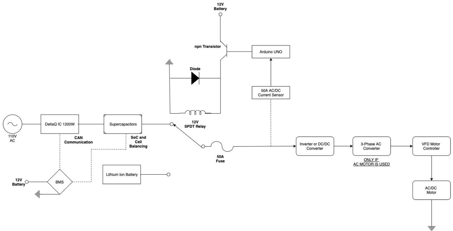
Figure 10: 2-D Electrical System Schematic of 2019-2020 Power Module.
