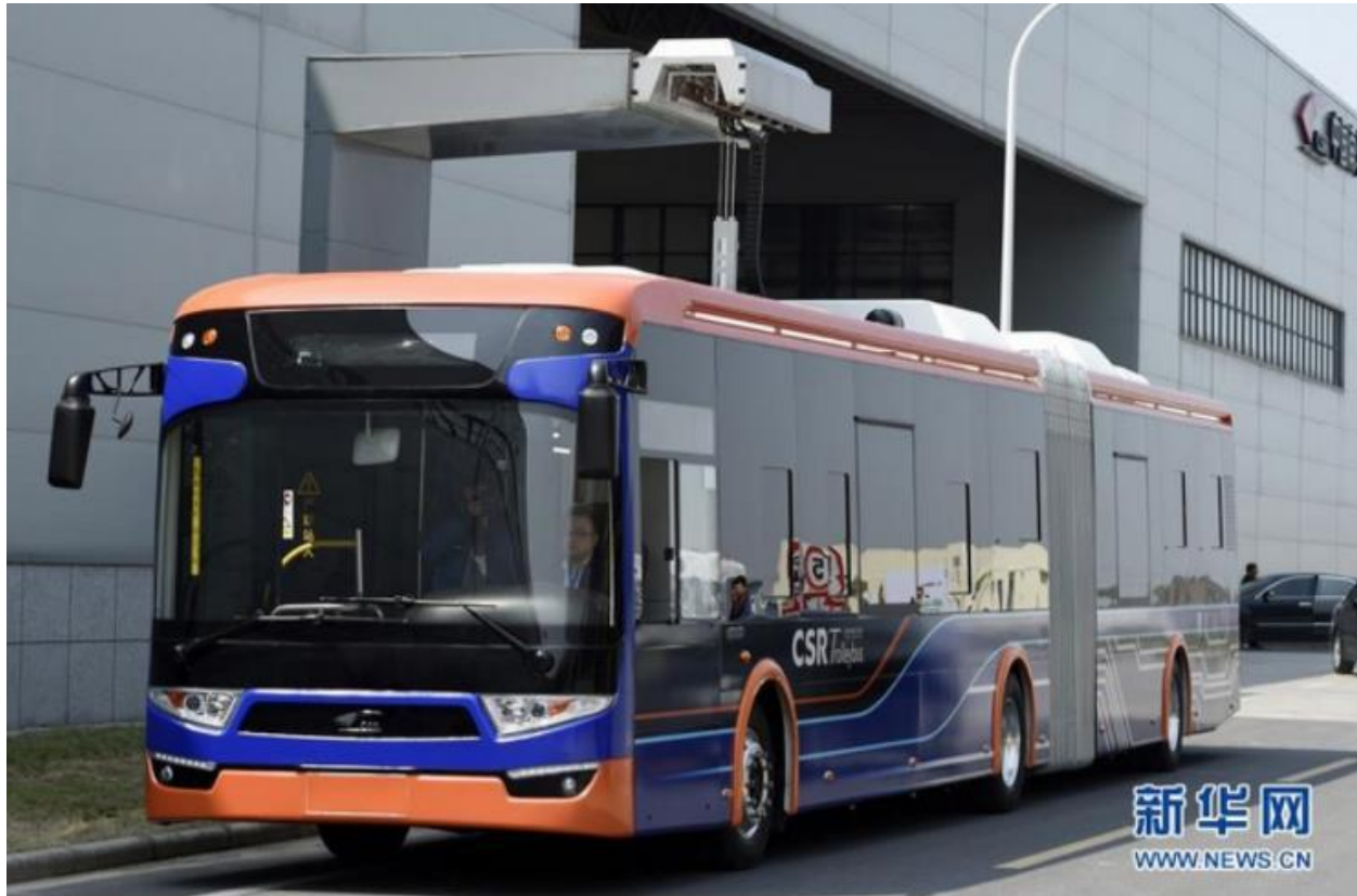
Rechargeable electric bus : 10 seconds to charge thanks to supercapacitors
