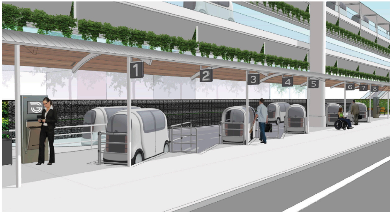
Figure C.5: Boarding Zone showing ticket kiosk and numbered individual boarding bays
