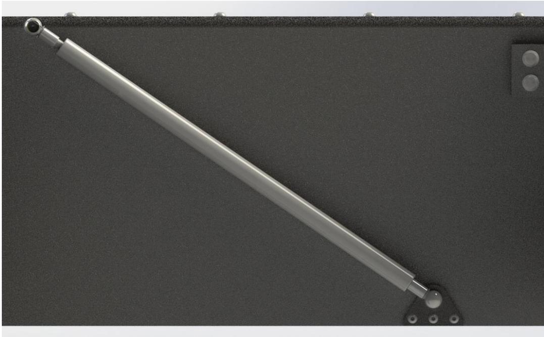
Figure 8. Gas spring setup. Two gas springs are mounted on the chute frame using ball socket end fittings and ball stud mounting brackets. These gas springs are used to force open the hatch as it is unlatched.
