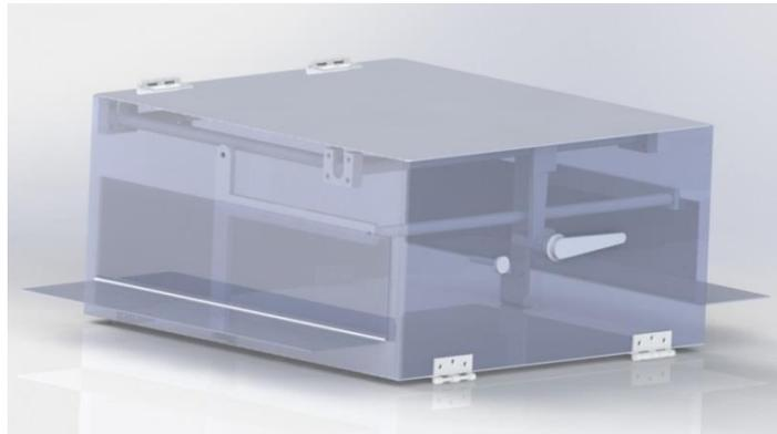
Figure 47. Second generation release mechanism. Twisting the handle of this unit releases the chute and unlocks the hatch. Passengers then have to open the hatch to gain access to the entry point.
