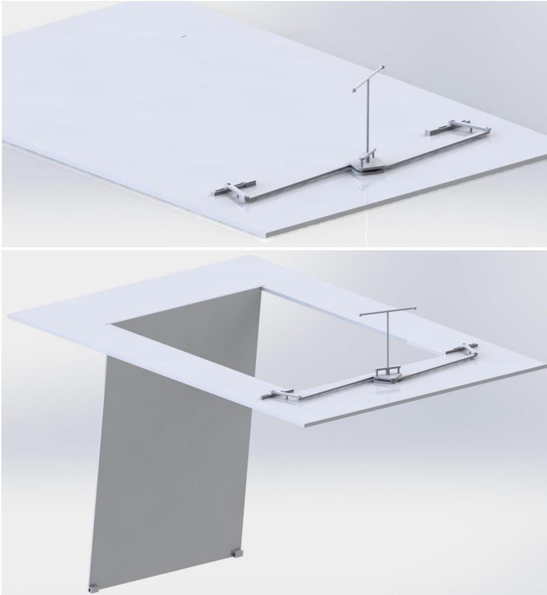
Figure 46. First generation release mechanism. These images represent the open and closed positions of one of the old release mechanisms. Twisting the handle unlatches the bottom door, and gravity forces the door open.
