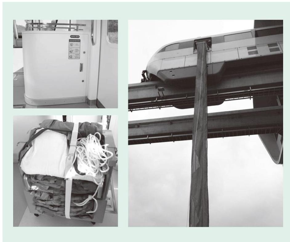
Figure 2. Hitachi Monorail emergency egress system (Kimijima, Kim, Furuta, & Sakatsume, 2017). Hitachi, a Japanese company, is using escape chutes for the emergency egress system of its monorails in South Korea.
