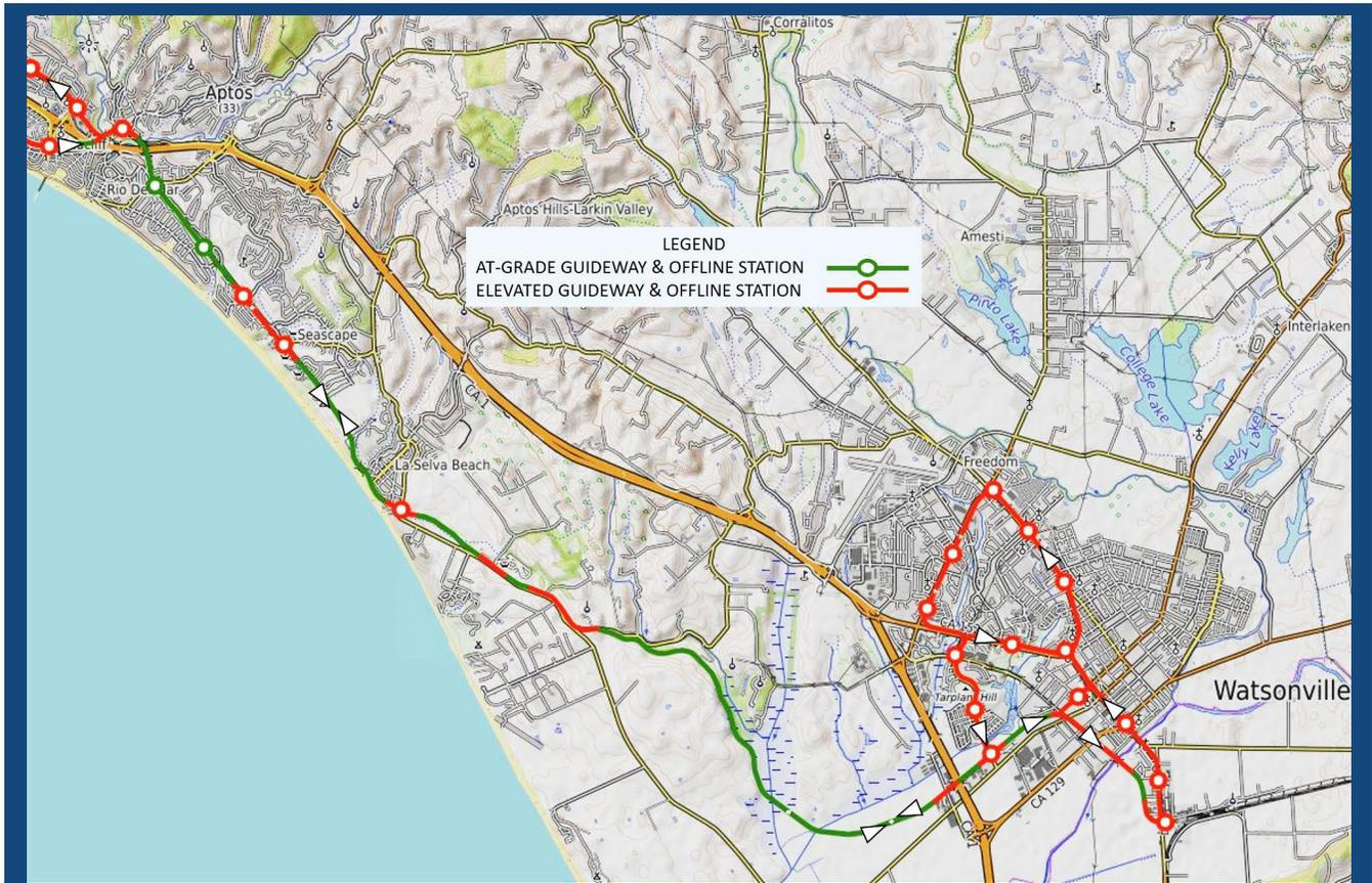
Figure 8. Conceptual ATN Layout Aptos to Watsonville
