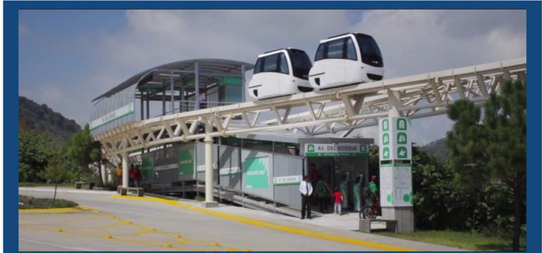
Figure 6. Modutram PRT Vehicles Leaving Station
