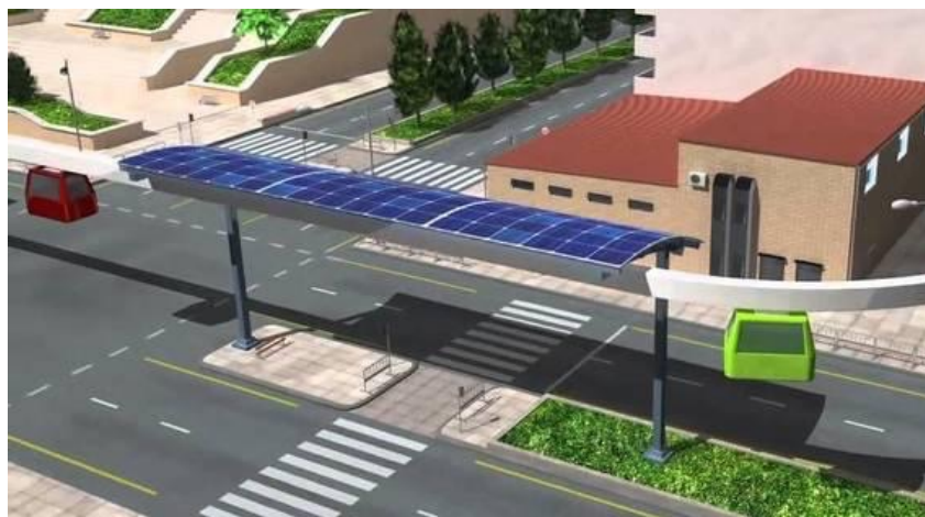
Figure 1. Solar Powered Automated Transit. Relatively small vehicles traverse a network of exclusive guideways and utilize off-line stations to provide on-demand, non-stop, origin-to-destination mobility. Suspending the ATN vehicle below the guideway makes the upper surface available for PV panels that can power the system. (JPods system, from (Wilmott, 2015))
