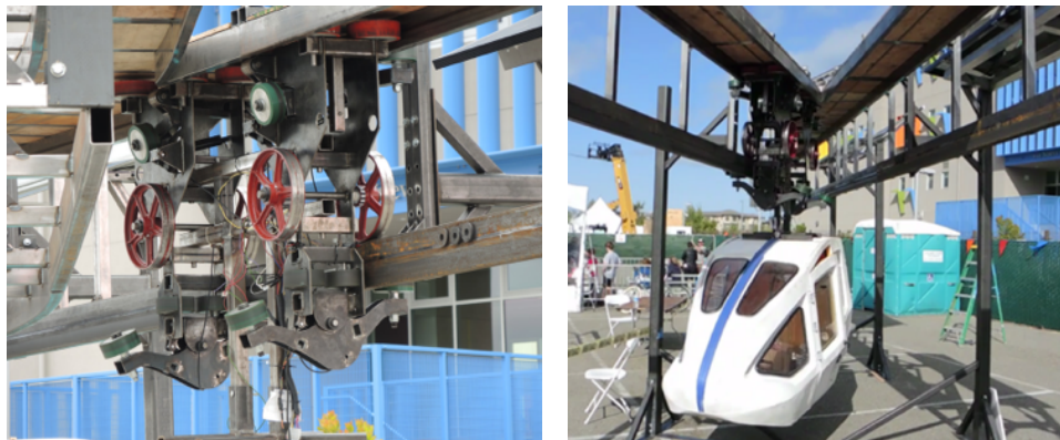
Figure 6. 2015 Full Scale Prototype. Motorized bogie and guideway section demonstrating switching ability at Maker Faire
