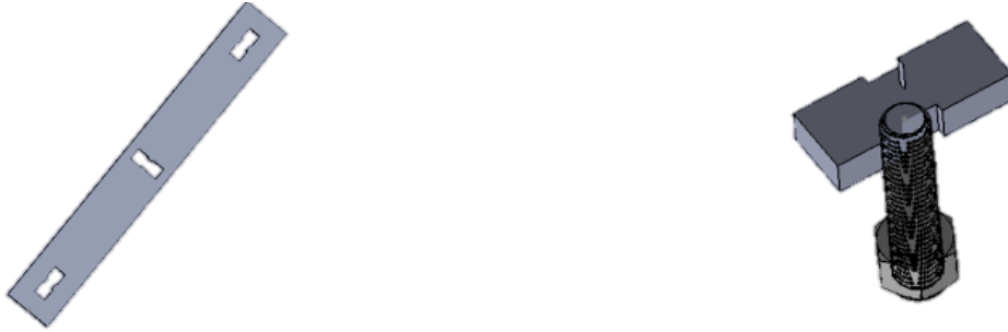
Figure 23: On the left is an extruded plate to fit the head of the CAM Lock located on the right.
