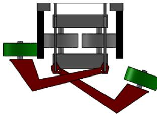
*Figure D-5: Single link for each wheel*
