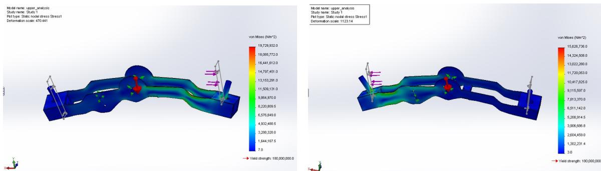
Figure D-9: Stress analysis of upper steering arm in both configurations
