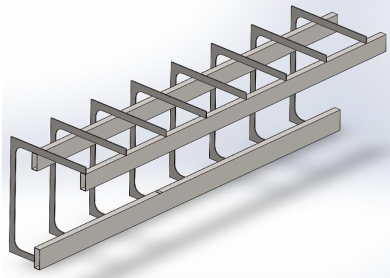
*Figure B-4: Iteration using tube steel for track instead of solid pieces*
