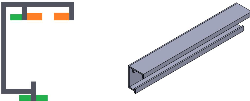
*Figure B-2: Revised Cross-Section and Isometric View for Track, Early Design Concept*
