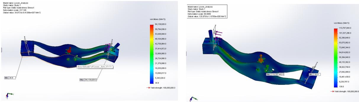
Figure D-11: Stress analysis of lower steering arm in both configurations.
