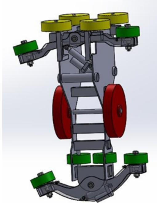
*Figure A-3: Bogie Switching Mechanism*
