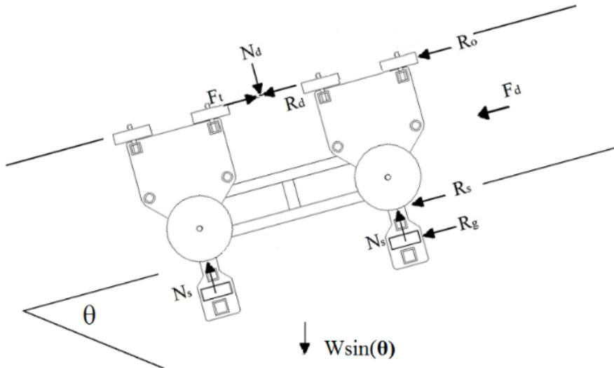
$$\sum F_x = m \times a = F_T - R_D - R_o - F_D - R_s - R_G - W \sin(\theta)$$
