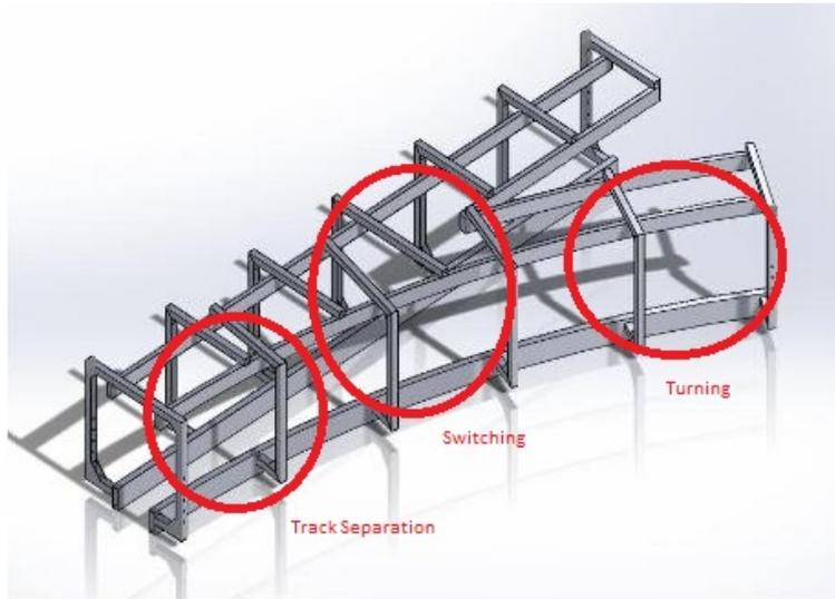
*Figure D-1: Critical locations for steering mechanism force analysis*
