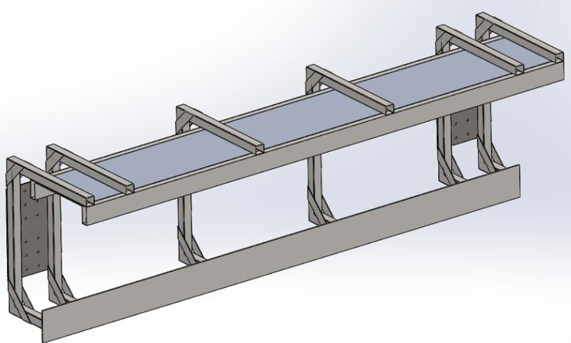
*Figure B-5: Nearly final iteration of guideway straight section*
