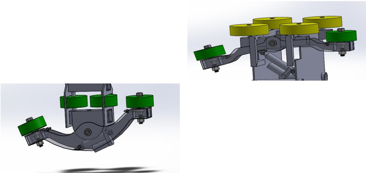
*Figure D-7: Upper (right) and Lower (left) switching mechanisms*
