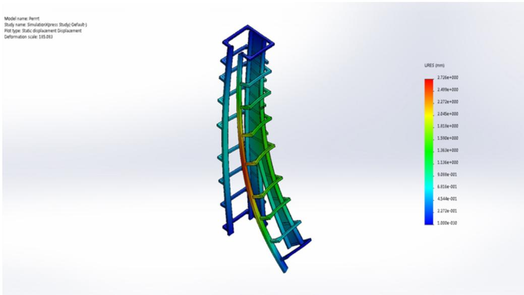
*Figure B-16: Curved portion critical loading (SF 1)*
