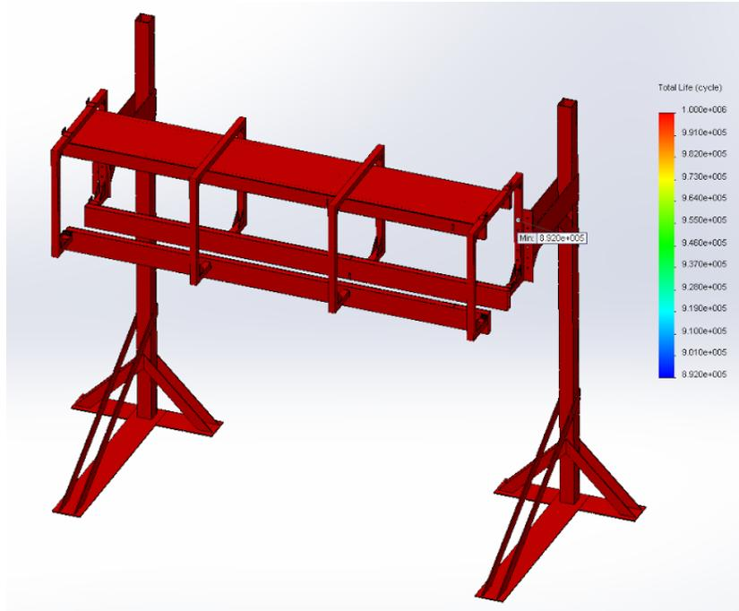
Figure B-E: Fatigue Analysis of Single Sided Straight Section
