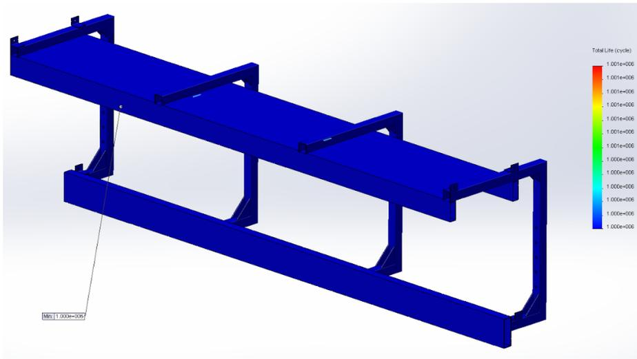
*Figure B-D: Fatigue Analysis of Single Sided Straight Section*
