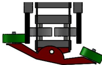
*Figure D-6: Single link for both wheels*
