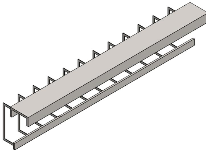
*Figure B-3: Iteration using “Ribs” to support track*
