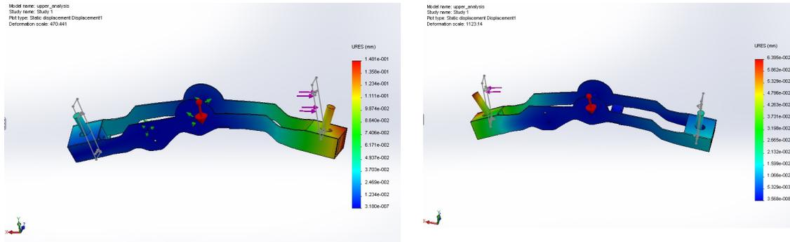
Figure D-10: Displacement analysis of upper steering arm in both configurations
