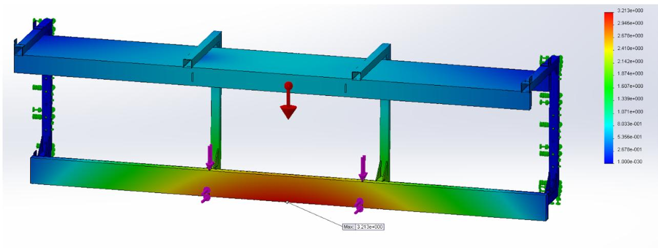
Figure B-B: Deformation of guideway at center position
