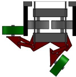
*Figure D-4: Four-bar steering mechanisms*
