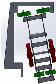
*Figure D-3: Bogie rolling off the guideway during cornering*
