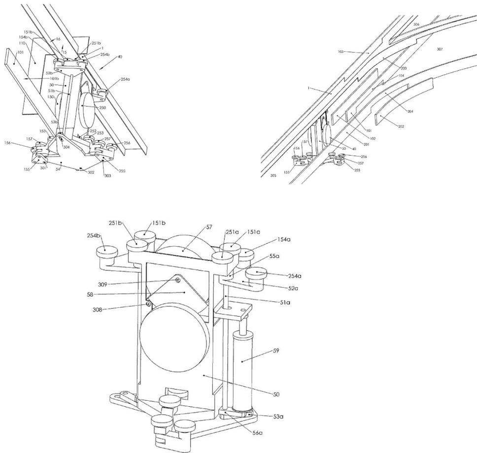
*Figure A-6: Track and Bogie for Suspended vehicles
