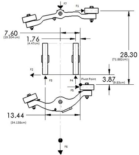
Figure D-A-A: Force analysis for track separation
