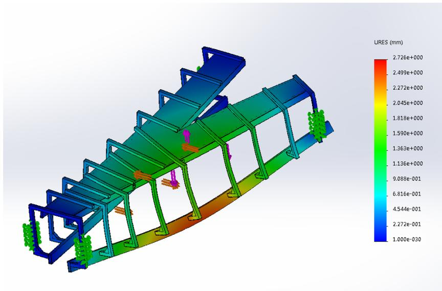
Figure B-15: Straight portion critical loading (SF 1)
