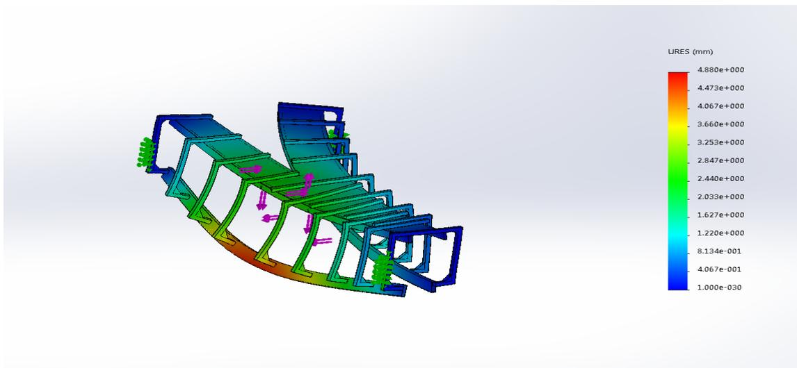
*Figure B-14: Straight portion critical loading (SF 2)*
