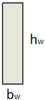
$$I_{wx} = \frac{b_w h_w^3}{12} \quad I_{wy} = \frac{h_w b_w^3}{12} \quad J_w = I_{wx} + I_{wy} \quad c_w = \frac{h_w}{2}$$
