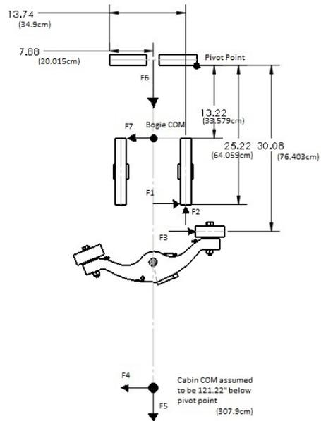
Figure D-A-C: Force analysis for cornering section
