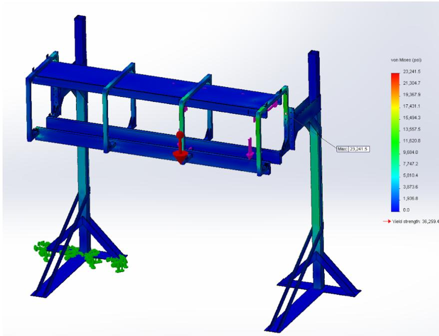
*Figure B-12: Static Loading of double sided section at worst loading configuration*
