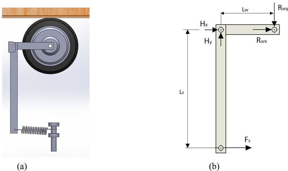
*Figure C-4: Unattached model of Prototype Propulsion System*
