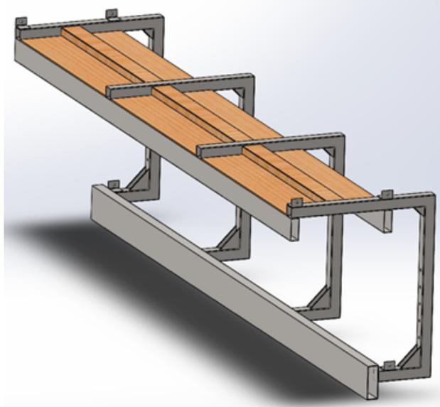
*Figure A-1: Single Sided Guideway Section*
