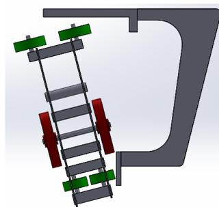
*Figure D-2: Bogie falling off guideway during switching*
