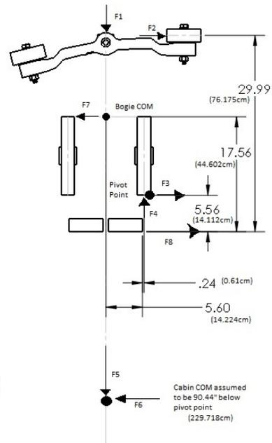
Figure D-A-B: Force analysis for switching section
