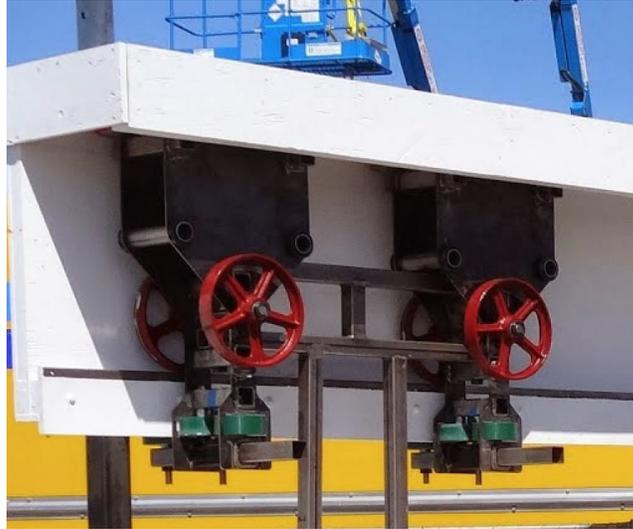
*Figure A-7: Full scale prototype for the bogie and guideway.*
