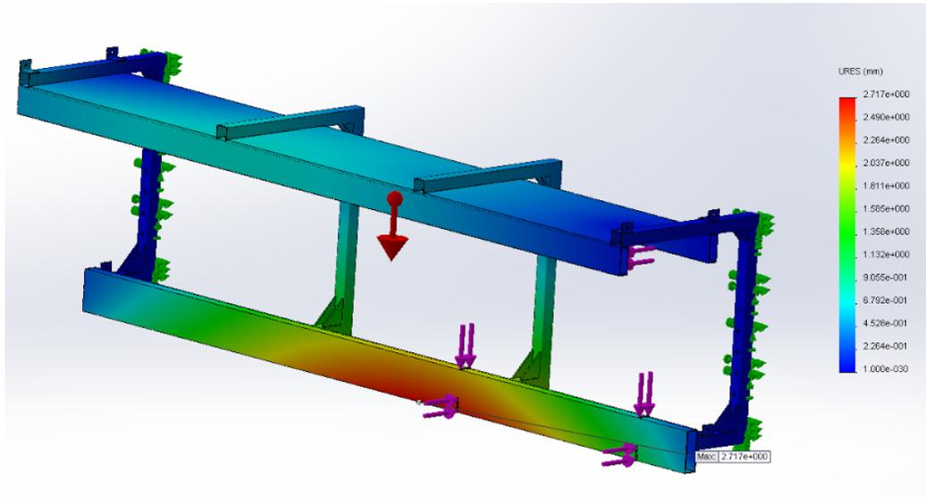
*Figure B-11: Relative deformation of guideway*
