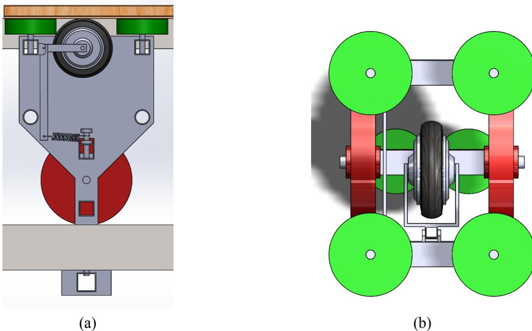
*Figure C-3: Model of Prototype Propulsion System installed on bogie
