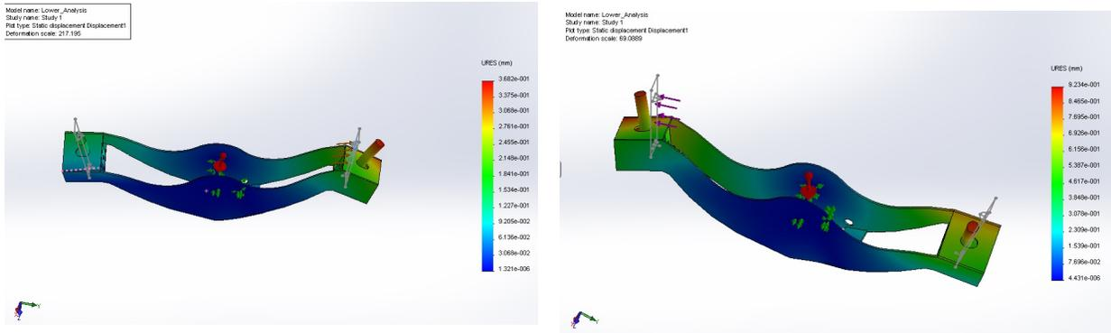
*Figure D-12: Displacement analysis of lower steering arm in both configurations*
