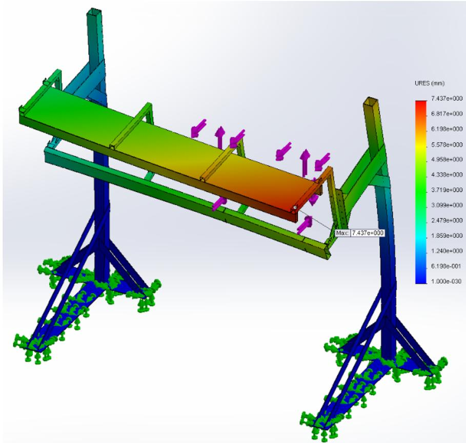
*Figure B-C: Total deformation of guideway*
