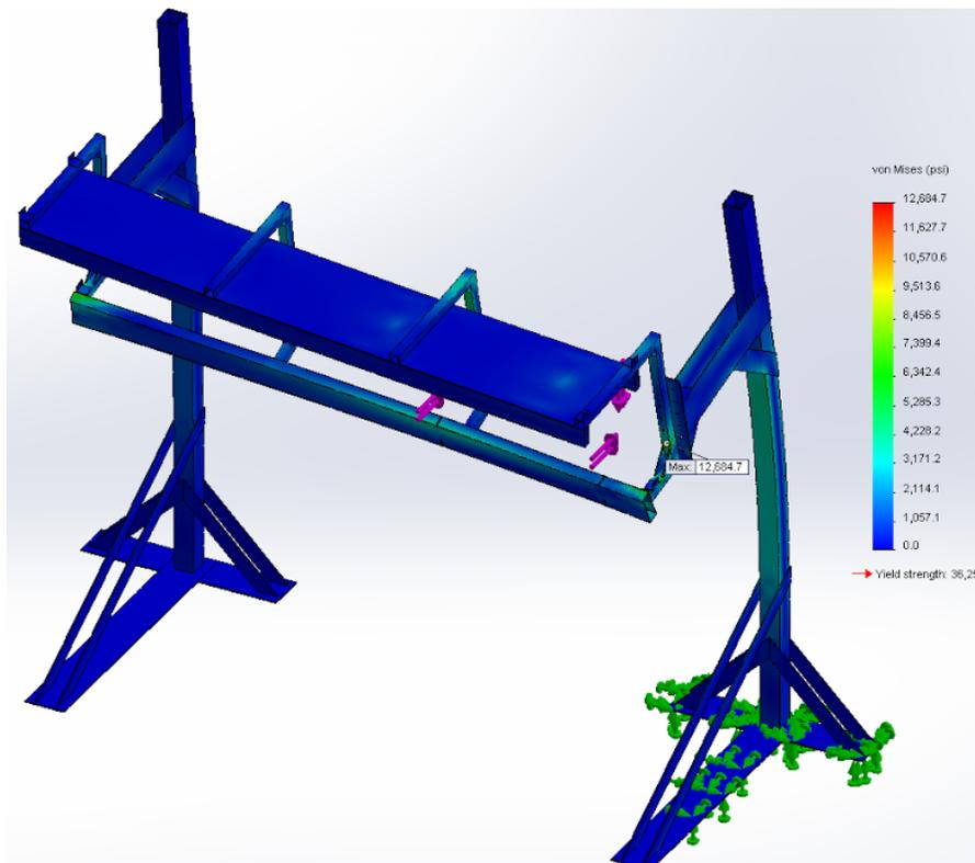
*Figure B-10: Static Loading at edge of Guideway Section*
