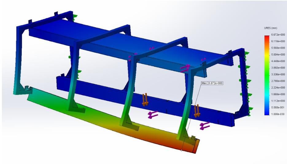
Figure B-13: Relative deflection for edge configuration of double sided guideway
