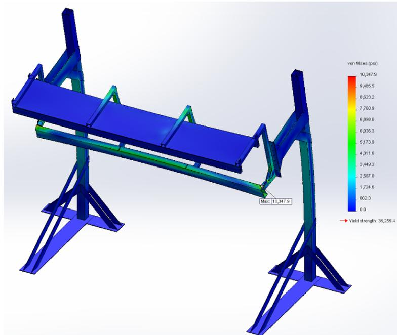
Figure B-A: Analysis of guideway at center
